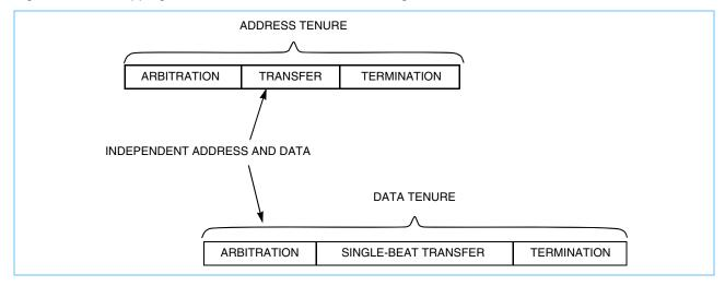
The basic functions of the address and data tenures are as follows:
