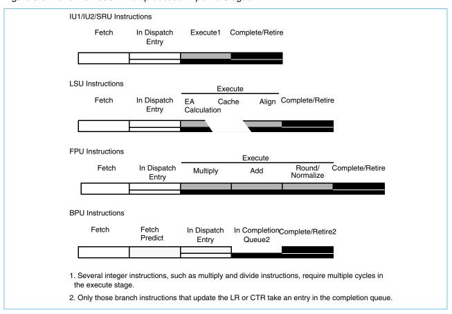
The 750CL's BPU decodes and executes branches immediately after they are fetched. When a conditional branch cannot be resolved due to a CR data (or any) dependency, the branch direction is predicted and execution continues on the predicted path. If the prediction is incorrect, the following steps are taken:
