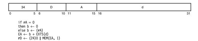
EA is the sum (rA|0) + d. The byte in memory addressed by EA is loaded into the low-order 8 bits of rD. The remaining bits in rD are cleared.
