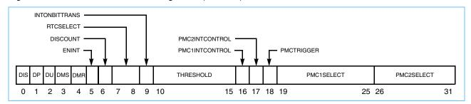
This register must be cleared at power up. Reading this register does not change its contents. *Table 11-2* describes the bits of the MMCR0 register.
