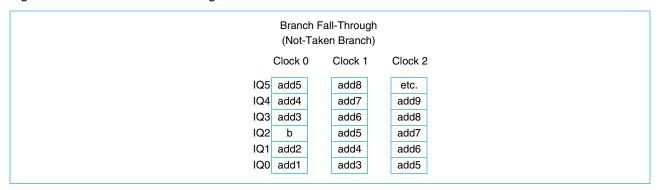
When a branch instruction is detected before it reaches a dispatch position, and if the branch is correctly predicted as taken, folding the branch instruction (and any instructions from the incorrect path) reduces the latency required for flow control to zero; instruction execution proceeds as though the branch was never there.
