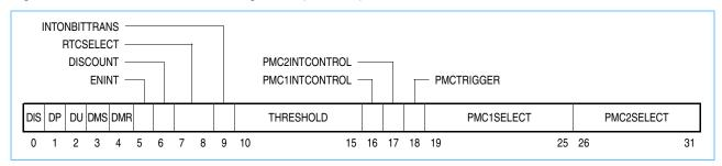
This register must be cleared at power up. Reading this register does not change its contents. The bits of the MMCR0 register are described in Table 2-9.
