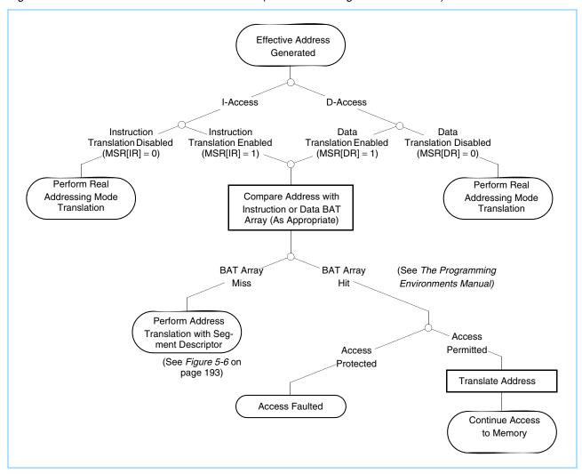
**Note:** If the BAT array search results in a hit, the access is qualified with the appropriate protection bits. If the access violates the protection mechanism, an exception (either ISI or DSI) is generated.
