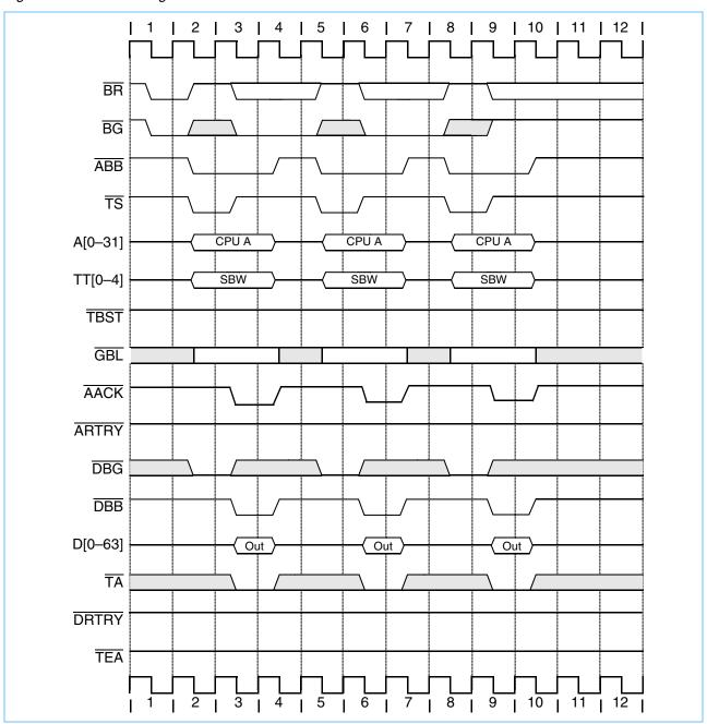
Figure 8-18 shows three ways to delay single-beat reads showing data-delay controls:
