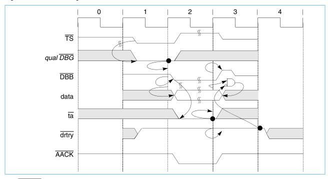
The DRTRY signal is not sampled during data writes, as shown in *Figure 8-11*.
