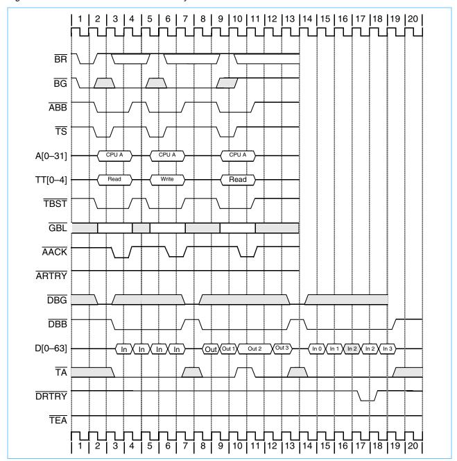
Figure 8-21 shows the use of the  $\overline{\text{TEA}}$  signal. Note that all bidirectional signals are three-stated between bus tenures. Note the following:
