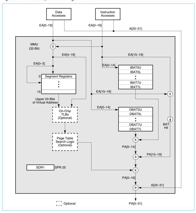
Figure 5-2. PowerPC 750CL Microprocessor IMMU Block Diagram
