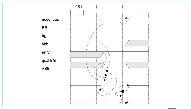
When the 750CL receives a qualified bus grant, it assumes address-bus mastership by asserting  $\overline{ABB}$  and negating the  $\overline{BR}$  output signal. Meanwhile, the 750CL drives the address for the requested access onto the address bus and asserts transfer start ( $\overline{TS}$ ) to indicate the start of a new transaction.
