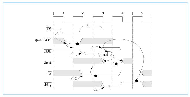
Figure 8-14 shows the effect of using  $\overline{DRTRY}$  during a burst read. It also shows the effect of using  $\overline{TA}$  to pace the data-transfer rate. Notice that in bus clock cycle 3 of Figure 8-14,  $\overline{TA}$  is negated for the second data beat. The 750CL data pipeline does not proceed until bus clock cycle 4 when the  $\overline{TA}$  is reasserted.
