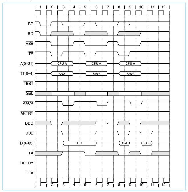
*Figure 8-20* shows the use of data-delay controls with burst transfers. Note that all bidirectional signals are three-stated between bus tenures. Note the following:
