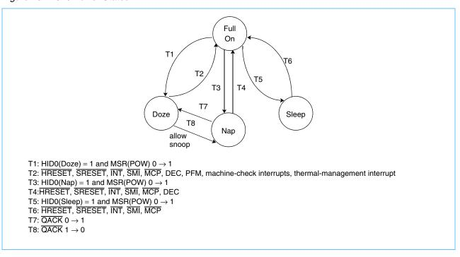
Hardware can enable a power management state through external asynchronous interrupts. Such a hardware interrupt causes the transfer of program flow to interrupt handler code that then invokes the appropriate power saving mode. The 750CL also contains a decrementer which allows it to enter the nap or doze mode for a predetermined amount of time and then return to full power operation through a decrementer interrupt.
