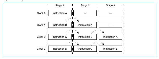
The 750CL can retire two instructions on every clock cycle. In general, the 750CL processes instructions in four stages—fetch, decode/dispatch, execute, and complete as shown in *Figure 6-2*. Note that the example of a pipelined execution unit in *Figure 6-1* is similar to the three-stage FPU pipeline in *Figure 6-2*.
