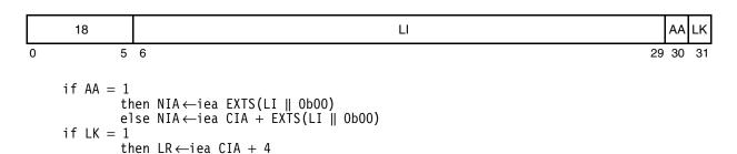
target\_addr specifies the branch target address.
